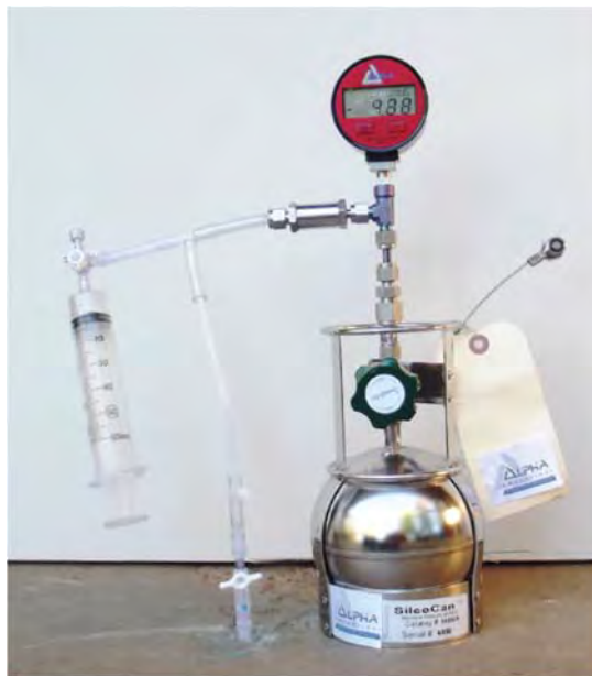
Figure 4: Vacuum leak check and sampling configuration
