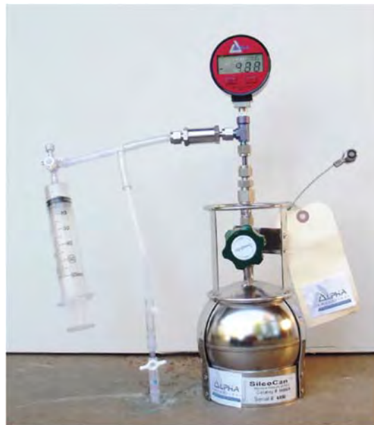
Figure 4: Vacuum leak check and sampling configuration
