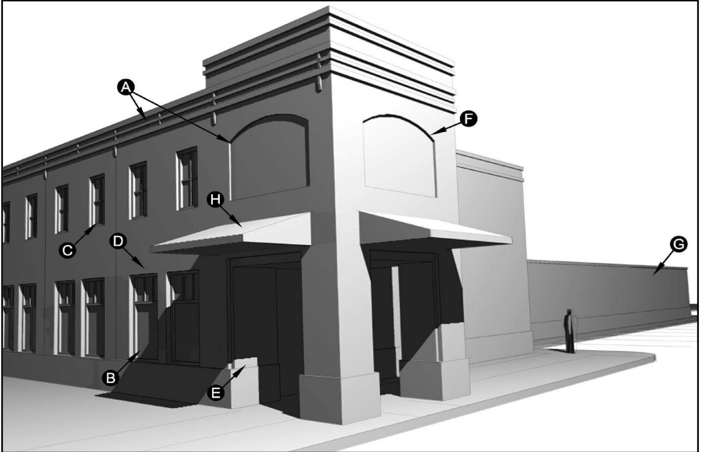
Figure G5.1: Fenestration is a Measure of the 3-Dimensional Depth of a Façade Created by Fluctuations or Openings in a Wall. Recesses such as archways or deep windows are two examples of fenestration. They help to give a façade a more 3- dimensional appearance by casting shadows and creating a visual contrast
