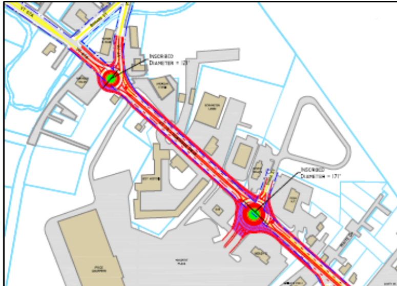
Suggested intersection improvements along the congested Route 7A/67A corridor include roundabouts at the intersection of those two highways and at the Monument Plaza intersection. (Northside Drive Roundabout Conceptual Design, 2006, by Resource Systems Group.) The proposed roundabout at the Monument Plaza intersection will be constructed as part of the Wal-Mart expansion.
