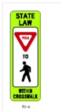
Figure 66 In-Street Crosswalk Sign
