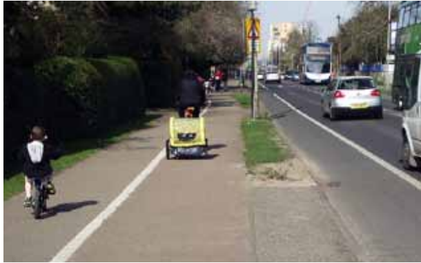
This path, separated from the road with a green strip, is comfortable and safe enough for children.
