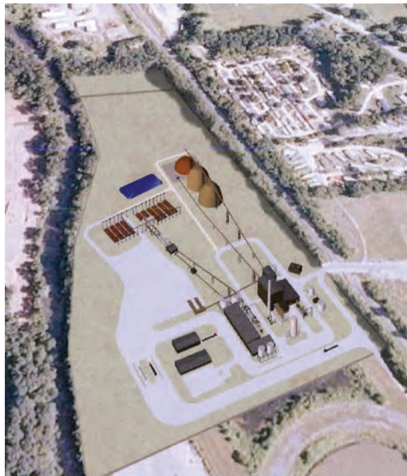
Site plan for a biomass-based electricity generating facility previously considered for a site in Pownal; waste heat from the process would be used in an on-site pellet manufacturing process. A similar project proposed for Fair Haven, Vermont, would also use excess heat to support a 10-acre greenhouse to supply year-round local food.
